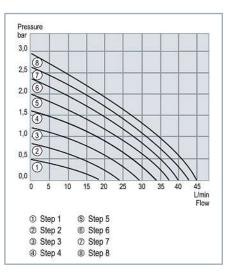
Characteristics of the vario pump of the Integral XT thermostat. The pump can be set in eight individual levels to adapt to a specific process, with a maximum pressure of 2.9 bar and a flow rate of 45 l/min.
